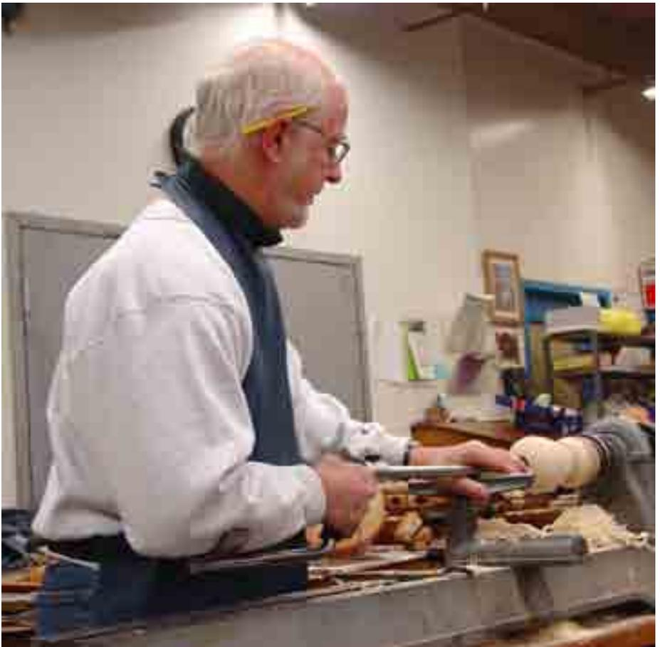
the initial drill hole all the way to the bottom of the vessel. I often alternate using the hooked tool and the straight tool until I have opened up a good sized hole to the bottom of the vessel.
