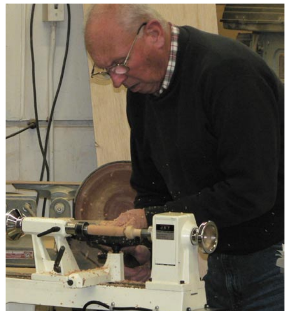
Turning a whistle, using the special mandrel.
