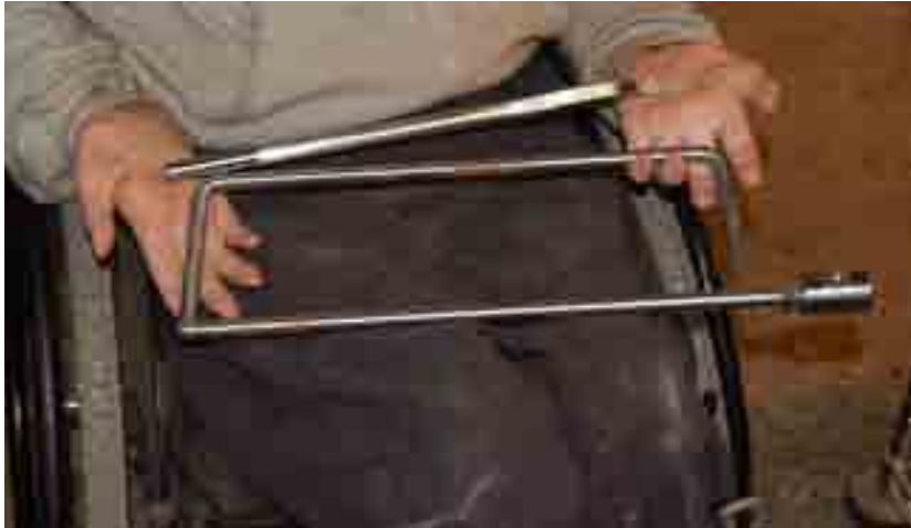
Custom-built handle for Kelton hollowing tool
