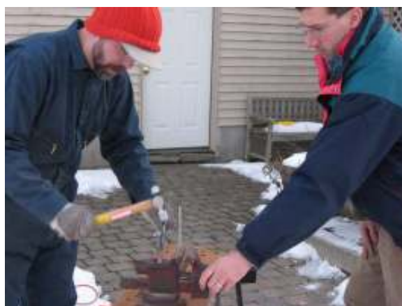
Shaping Red-Hot Tool Steel
