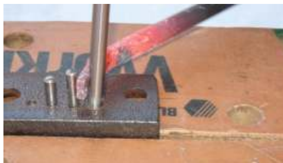
Shaping Red-Hot Tool Steel
