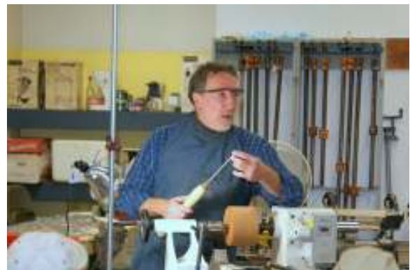
the glued-up stock is ready for turning with a bowl gouge with swept back wings.
