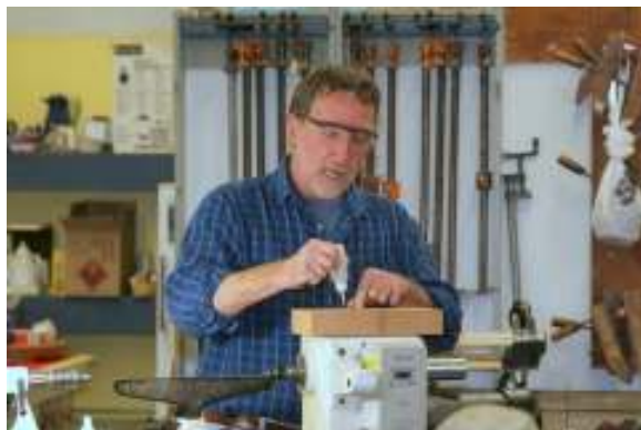
tack-glued with cyanoacrylate (super) glue...
