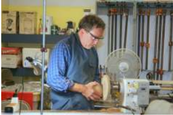
Sanding a base with a disk sander (traveling model).
