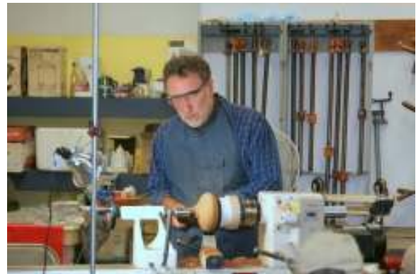
used as a jam chuck allows Al to nearly complete the other side.
