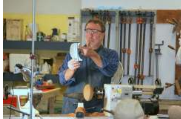
Using a profile gauge, Al gets a view of the profile after he removed the tenon from one side.
