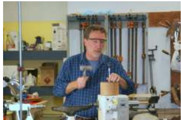
cut round on a bandsaw and centers marked gets you ready for turning.
