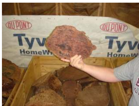
A gorgeous piece of Gimlet. Most of the dark spots are pitch pockets, which Rob explained can cause sparks to fly from the chainsaw when cutting.
