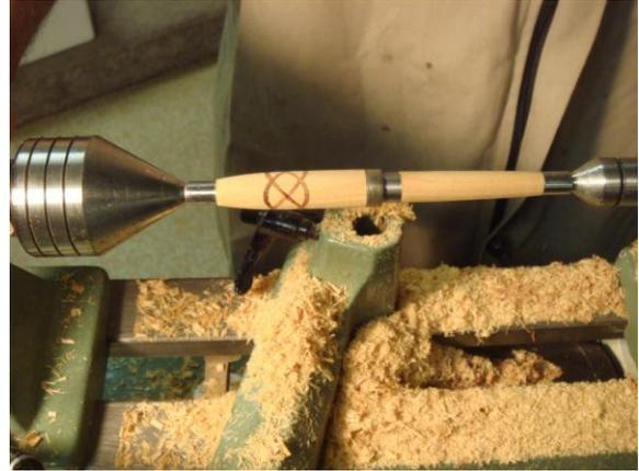
The two barrels mounted on bushings between centers—completed.
