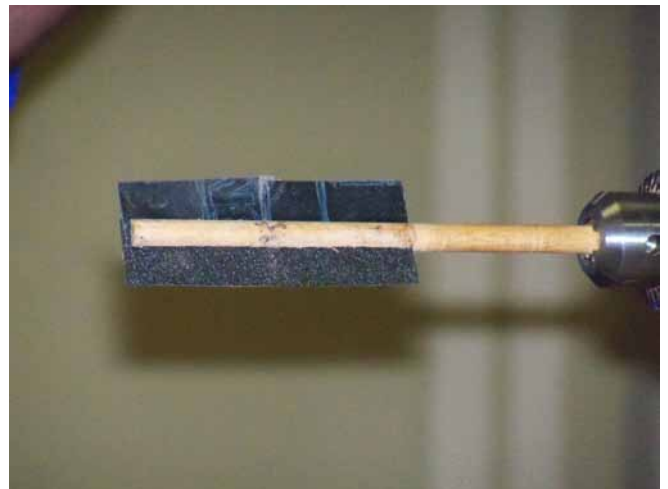
Home made tool for inside sanding
