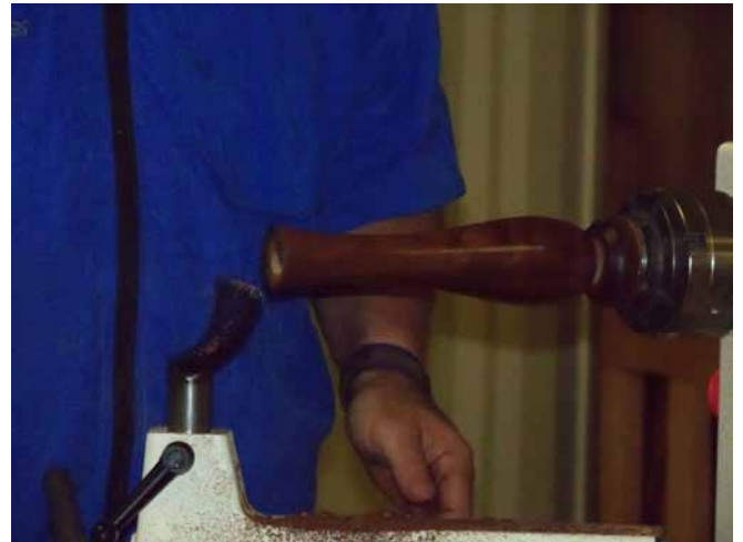
Vase has been sanded, polished and then drilled
