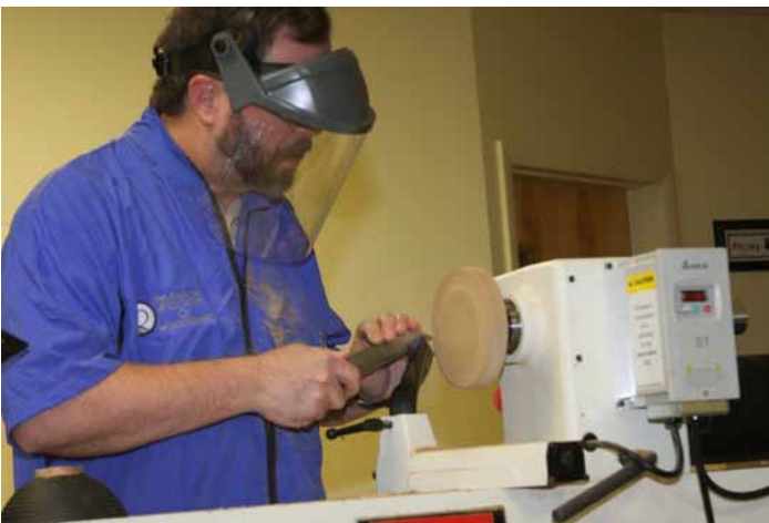
Making a jamb chuck to hold a bowl by the rim.
