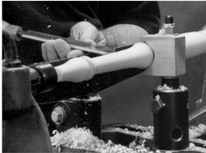
A mechanical steady rest in use
