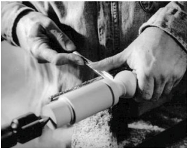
Using the hand to steady vibration
