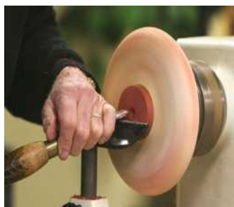
Turning hole in plug with sharpened point gouge
