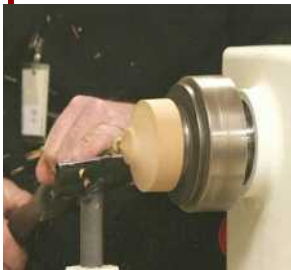
Turn a cone shape as a mandrel to fit into top
