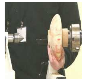
Mount vessel between mandrel and live center
