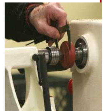
Checking diameter of tenon on bloodwood plug
