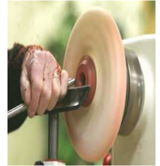
Shaping a collar with a 3/8 gouge
