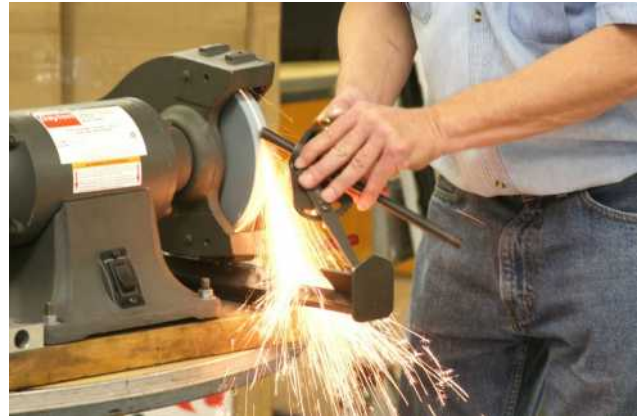
Doug recommends Norton 3x "k" wheel Nose angle 60° for bowl gouges
