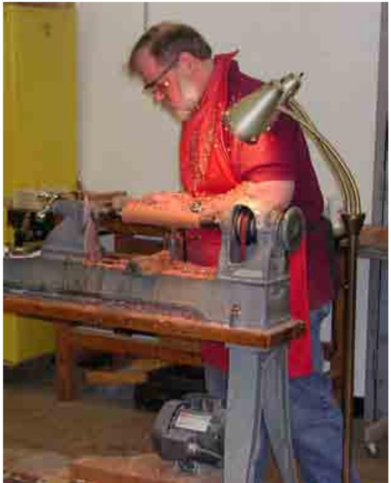
On most turnings I can just start from left to right, but some thin turnings work better to turn the center first and work outward a little to each side at a time. This keeps more material to the outside for stability.
