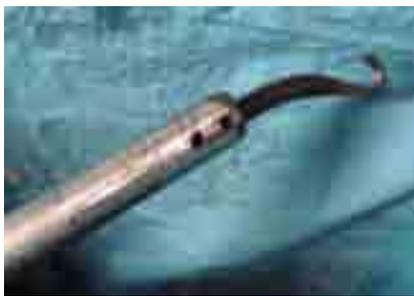
shaft for mounting such as the Wolok Hook Tool shown here. If the bit were not held firmly by the rod as shown it would be of little use. Once we have a steel rod holding the small bit we are then able to use the tool just as it is or, as is often done, with the other end of the rod inserted into a wooden tool handle such as would be typical of any other woodturning tool.
