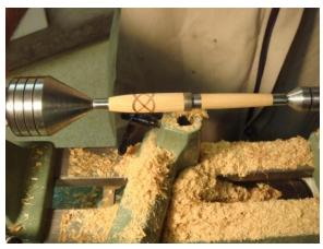
The two barrels mounted on bushings between centers—completed.
