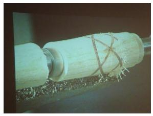
With a deft and clean cut with a skew chsel, the knot pattern is revealed.
