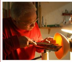
I will demonstrate how to use a conventional bowl gouge to turn a bowl with 1/16" wall thickness, using green wood and a light source to gauge the wall thickness. If you are
